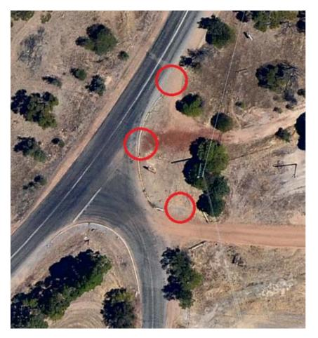
Barrier kerbing should not be used on high speed roads as it has the potential for vehicles to lose control, particularly motorcyclists, if struck.
