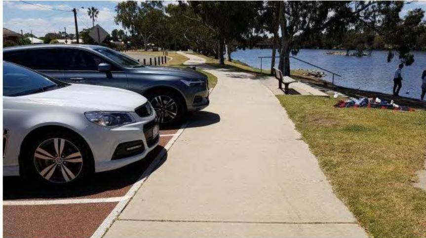
Photo 18: Lack of wheel stops means parked cars become a hazard to path users.
