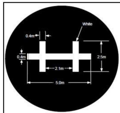
Figure 9: Glider Operations Signal
