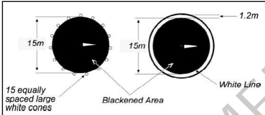
Figure 6: Options for Primary Wind Direction Indicator
