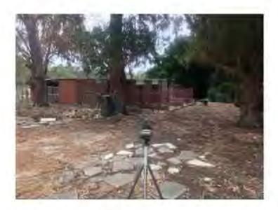
At the time of placing the logger, more detailed 1/3 octave band measurements where taken to ascertain the tonal characteristics of the dogs barking. In addition dB(A) measurements were taken for comparison with the noise logger results. It was observed that the main noises present during measurements were birds chirping, leaves rustling and the traffic of Great Eastern Hwy.
