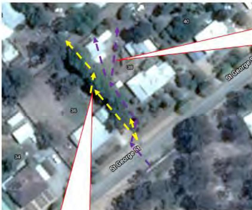
Altered flow path causing flooding to 38 St George Street (Current Situation)
