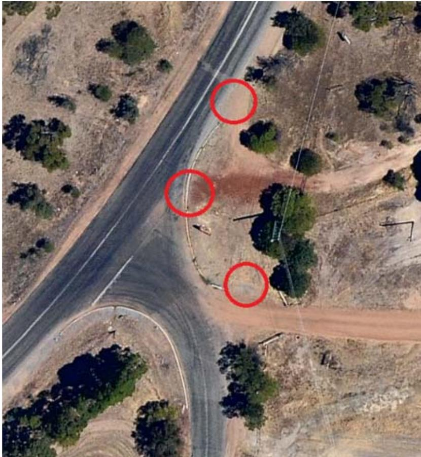
Barrier kerbing should not be used on high speed roads as it has the potential for vehicles to lose control, particularly motorcyclists, if struck.
