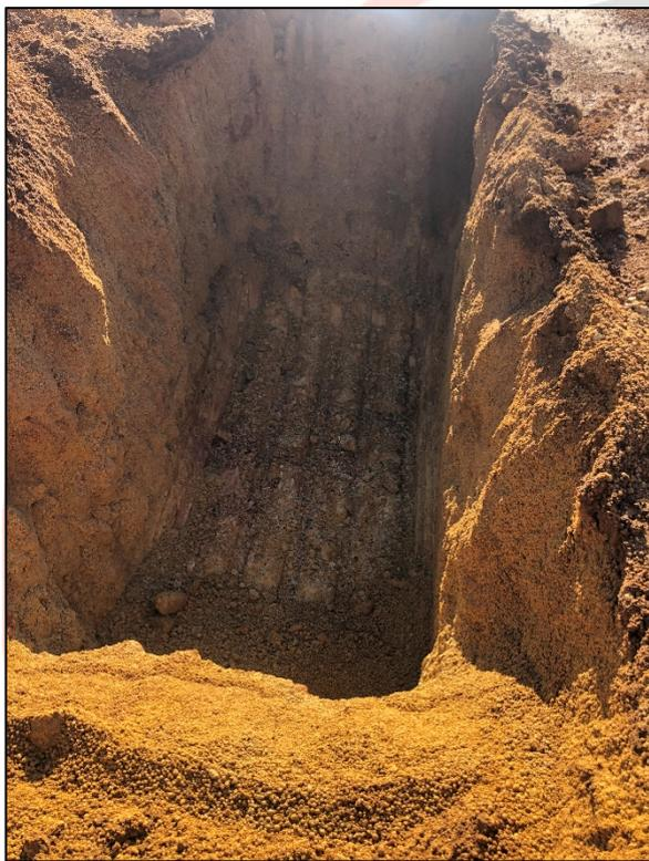
Photo 1: Excavation showing gravel, clay and laterite
