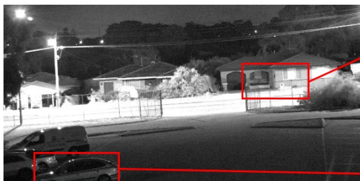
Poor Dynamic Response – unable to cater for highlight and low light conditions as well as generating excessive noise.
