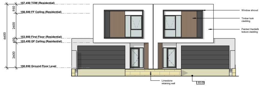
1 ELEVATION (FITZGERALD ST WEST) 1001 SCALE: 1 : 100
