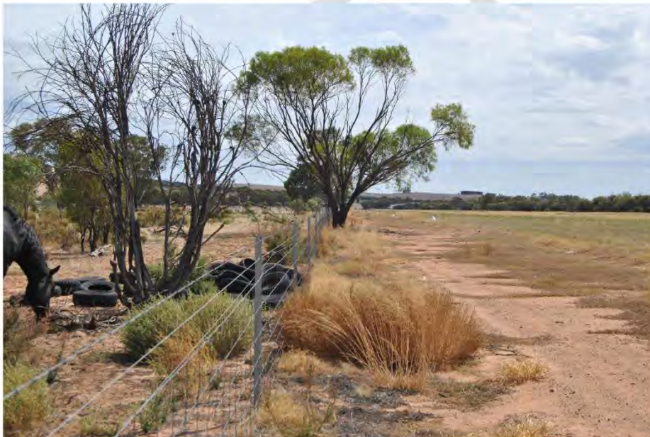
View facing north-west along the airport perimeter fence. The runway strip edge cones can be seen. Trees may infringe the transitional surface and should be assessed by survey to ensure the flyover areas are clear.
