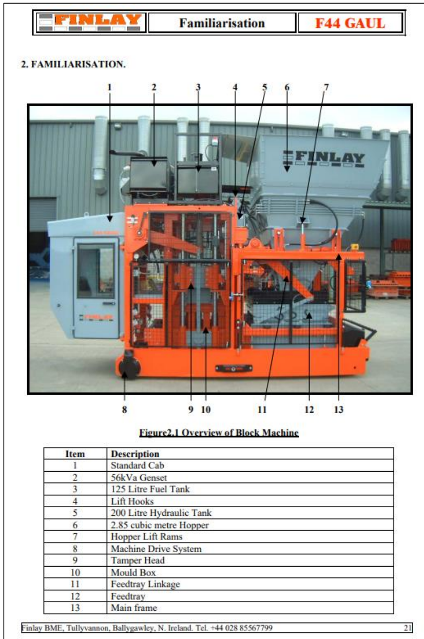
Figure 6: Finlay block machine specifications
