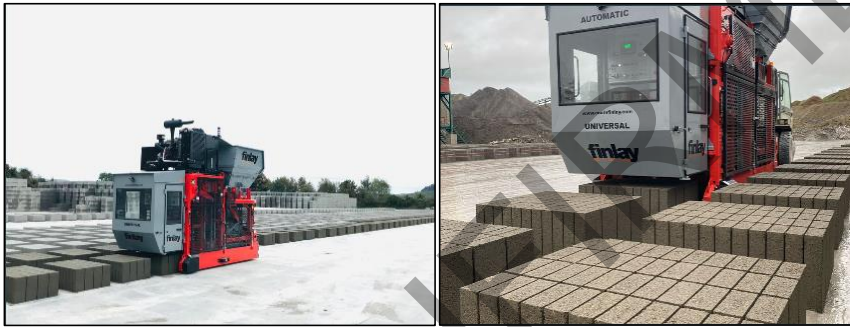
Photo 2: F44 block machine & typical block types
