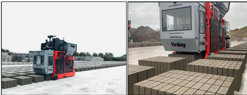
Photo 2: F44 block machine & typical block types
