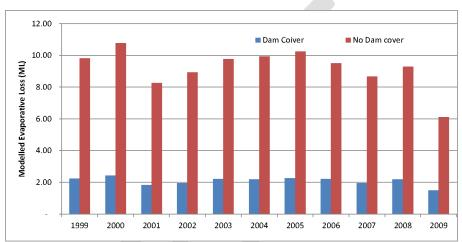
Figure 7. Impact of dam cover on the annual estimate evaporation.
