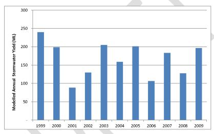
Figure 2. Modelled Annual Stormwater Discharge - Wundowie
