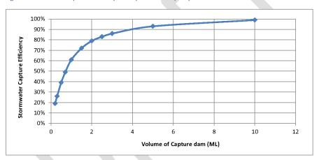
Figure 4. Stormwater capture efficiency and capture basin capacity
