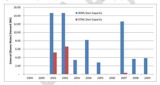
Figure 6. Annual External (scheme water) demand – for 30ML and 37ML storage dam capacity.
