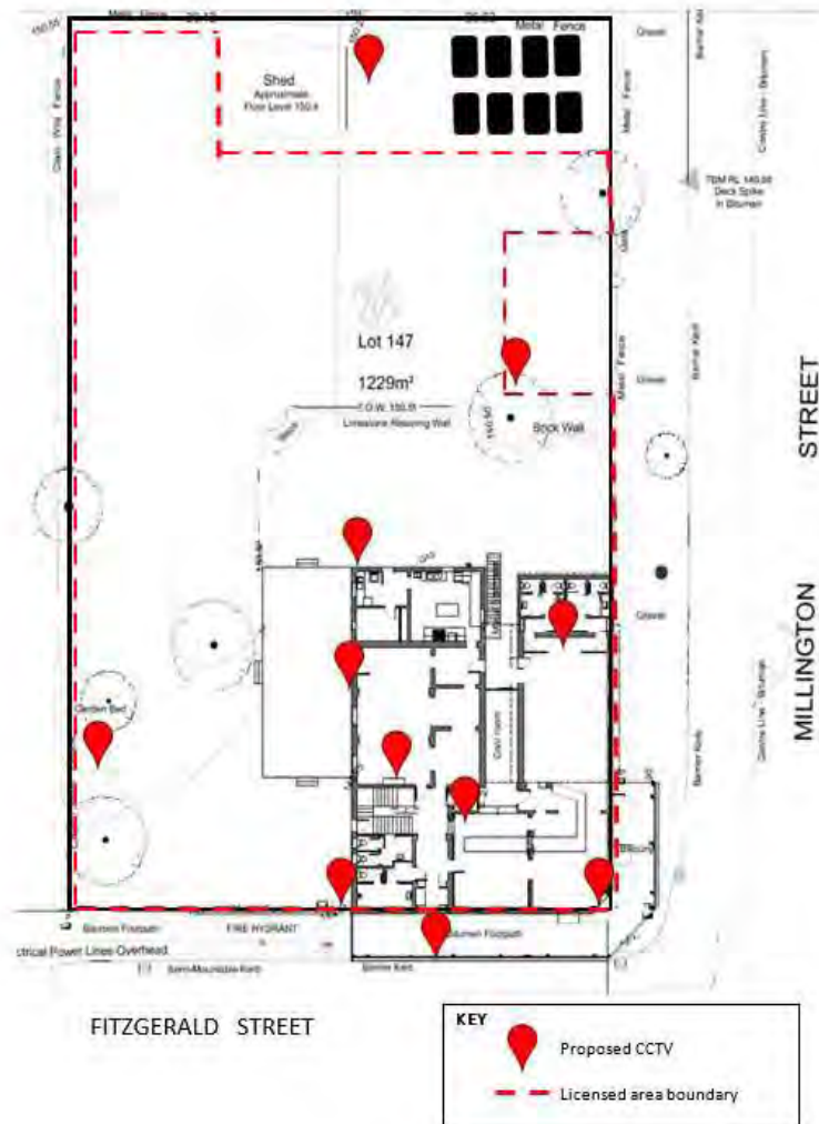
Figure 13 Proposed CCTV installation
