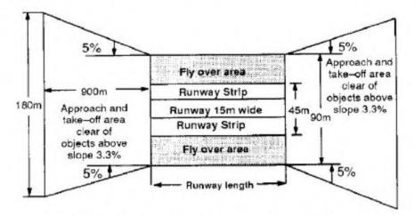
Figure 1 below represents the CAAP 92 basic guidelines for ALAs with operations during the hours of darkness.
