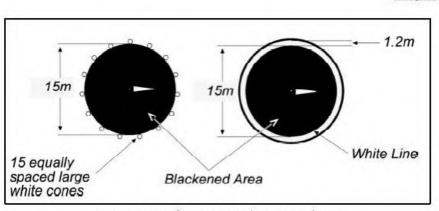
Figure 6: Options for Primary Wind Direction Indicator
