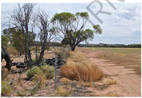
View facing north-west along the airport perimeter fence. The runway strip edge cones can be seen. Trees may infringe the transitional surface and should be assessed by survey to ensure the flyover areas are clear.
