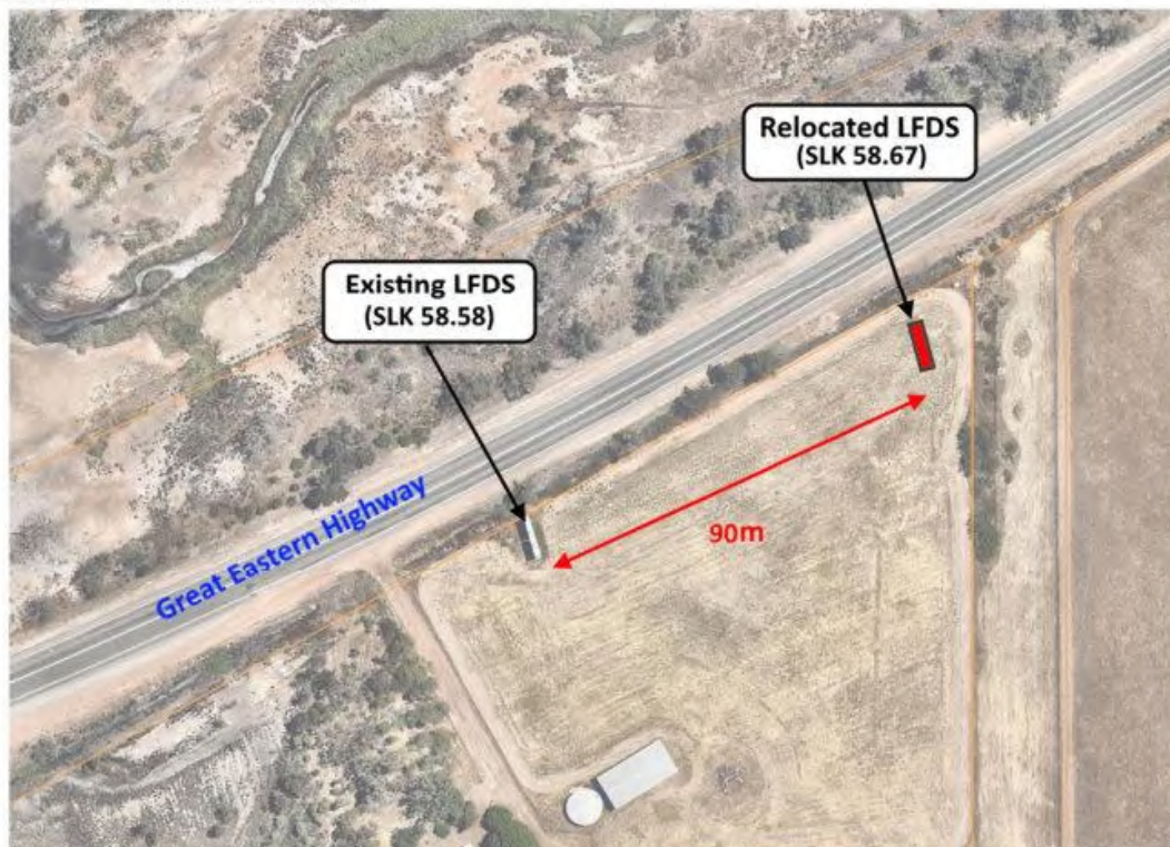
Figure 2-1 Relocated LFDS Position
