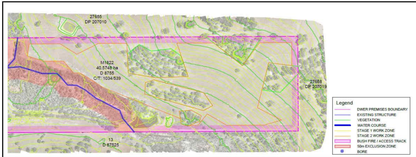
Figure 3: DWER Prescribed Premises boundary (pink thin line), surveyed and mapped water course mid line (blue line), 20 m boundary set back and bush fire / access track (shaded pink area) and 50 m exclusion zone from mid-line of the water course (red shaded area) for Stage 2 extraction area
