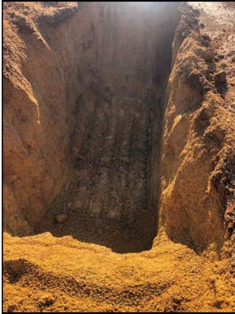
Photo 1: Excavation showing gravel, clay and laterite
