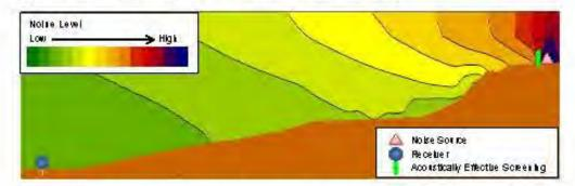
Based on the topography and plant location information provided by the Applicant, our calculations identify that screening in the locations identified in Figure 4 would need to be approximately 3.5 m high (or approximately 1 m higher than the noise generating element of the plant) in order be sufficient to block the line of sight between the plant and both receivers and, therefore, acoustically effective.
