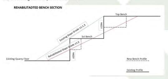
The only blasting that will occur will be make the existing benches safe and reduce the bench levels/heights to accommodate the reduced slope.
