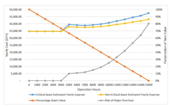
Figure 2: Cost vs Operating Hours for a critical and non-critical equipment
