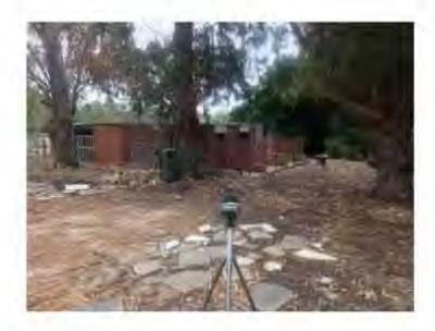
At the time of placing the logger, more detailed 1/3 octave band measurements where taken to ascertain the tonal characteristics of the dogs barking. In addition dB(A) measurements were taken for comparison with the noise logger results. It was observed that the main noises present during measurements were birds chirping, leaves rustling and the traffic of Great Eastern Hwy.
