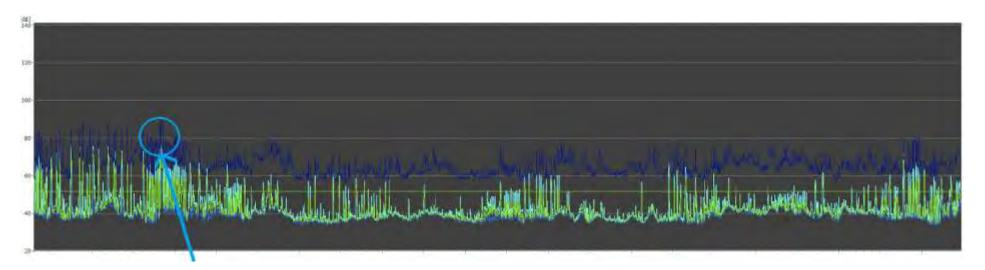
This spike in the Measurements indicates the point in Time where the owner left the property. This is the only time that the dogs were barking during the measurements for that day. All of the other spikes in the Sound Pressure Level (SPL) logging is attributed to Birds chirping in close Proximity the SPL meter.
