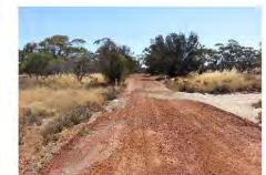
Road Hierarchy: Access Road RAV Route (Y/N): NO Bus Route (Y/N): Proposed Shire Focus (RRG): Trigger source: ICS Ranking: **Proposed Works:** Widen road for buses and culvert installation at floodways New culvert crossing with Associated Works: embankments to avoid flooding. Treatment cost: \$1,971,164
