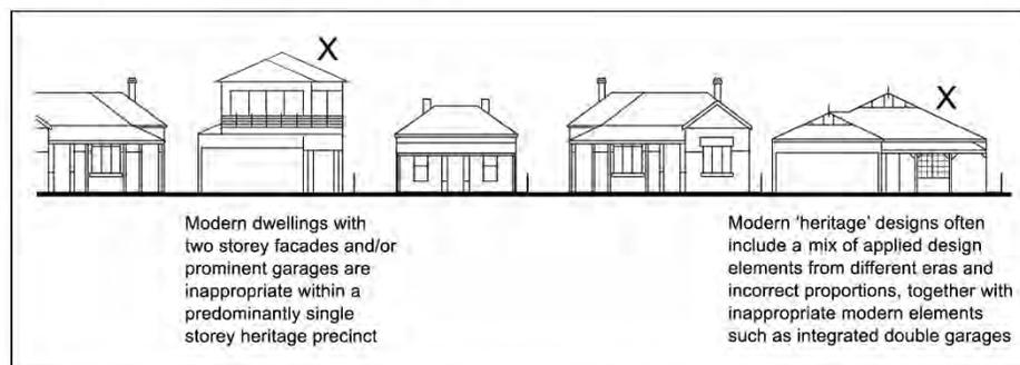
**Figure 5: Examples of inappropriate infill within a heritage precinct** (Indicative sketch only)
